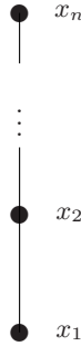
Fig. 4.5. Hasse diagram of a total order on S = \{x_1, x_2, \dots, x_n\} .
